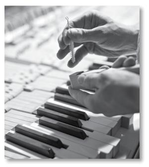
must be able to bear 20 tonnes of tension. Then there are 88 keys to be balanced, the hammers to be 'voiced' and the strings tuned.
