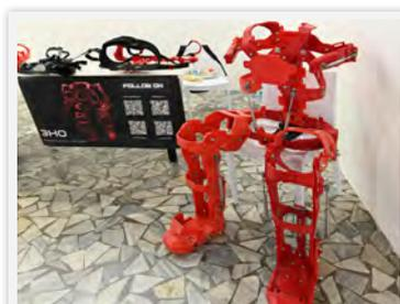
3D-printed exoskeleton prototype
